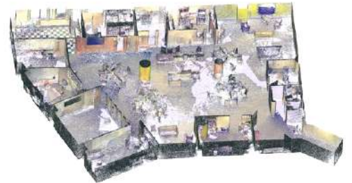
Color point cloud of commercial office space - note detail of wall colors and flooring
