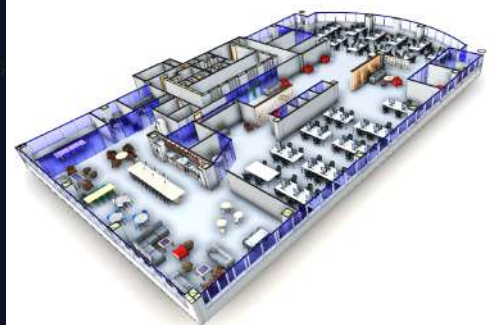
Scan to BIM for office project: Point cloud (left) captured by one person in 40 minutes. 3D BIM model created in Revit.
